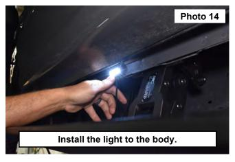
14. Secure all wires from any moving parts using the supplied wire ties, make sure all lights and steps are in working order. **See Photo 15.**
