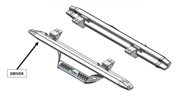
**Step. 2** Starting with the passenger side step rail, install the supplied (x4) 5/16" snap nuts into the two notches in each mounting bracket.
