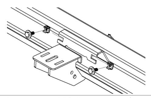
**Step. 7** After finial positioning, tighten all (x4) ¼"x ¾" hex bolts no more than 6 ft/lbs. torque.
