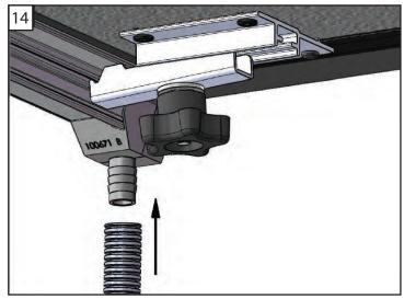
14. Attach the drain tubes to the fittings at the front of the bed rail and position the tubes to divert water out of the truck bed. This can be done by inspecting the area below the bed floor and drilling a 5/8" hole in the corner of the wheel well OR through an existing hole in the bed, enlarging it to 5/8"- Careful to not drill too far.
