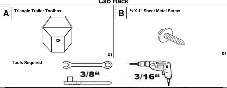
Position the triangle trailer toolbox (A) onto the trailer tongue of your trailer. Drill four 3/16" holes through the bottom of the triangle trailer toolbox (A) and the trailer tongue.
