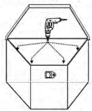
Secure the triangle trailer toolbox (A) to the trailer tongue of your trailer using the provided 1/4 x 1" sheet metal screws (B). Tighten into place using a 3/8" wrench / socket.
