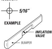
Install inflation valve assembly as shown.
