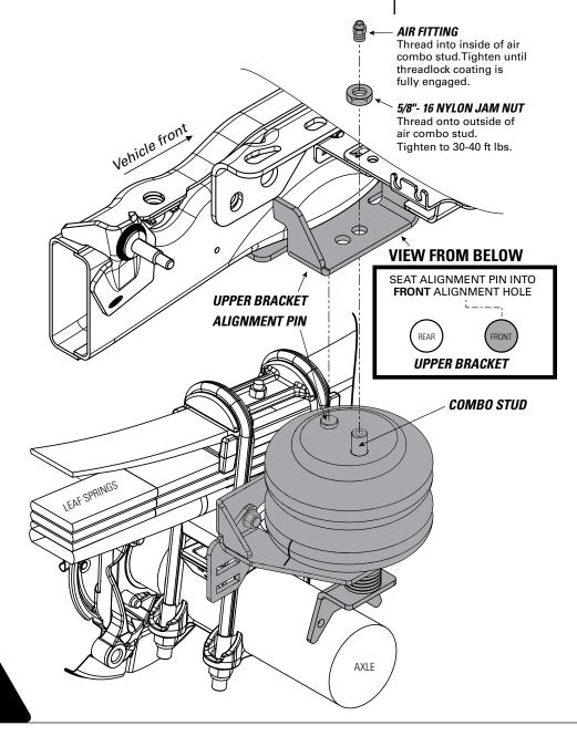
ALIGNMENT PIN ON AIR SPRINGS MUST BE INSTALLED TO FULLY SEAT INTO THE FRONT ALIGNMENT HOLE IN THE UPPER BRACKET. FAILURE TO DO SO WILL CAUSE IT TO BE PUSHED INTO THE BEAD PLATE, CREATING AN AIR LEAK, AND RESULTING IN AN AIR SPRING FAILURE THAT IS **NOT WARRANTABLE**. **THE ALIGNMENT PIN CANNOT HOLD 2,500 LBS! IT IS USED FOR ALIGNMENT ONLY!**
