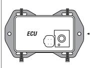
If there is no other mounting option, use two large Nylon ties to secure ECU to the location determined in planning the install section. Route the Nylon ties under the ECU and around the mounting location.
