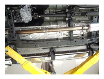
Step 3. Next, attach the Extension Pipe Assembly and the Muffler using the supplied 3.00" clamps and engaging the hanger into the rubber insulator.
