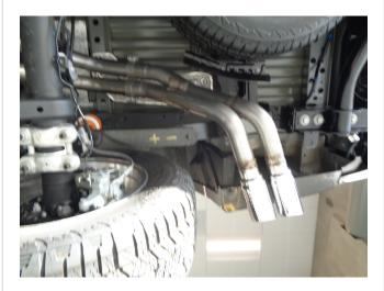
Step 5. Finish the installation by attaching the Tail Pipe Assembly to the Over Axle Pipes using the supplied 2.50" clamps and fitting the hanger into the rubber insulator.
