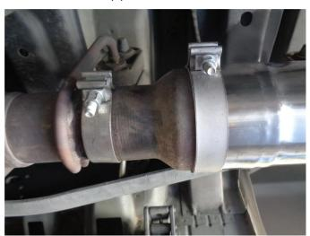
**Step 3.** Begin installation by loosely attaching the Inlet Pipe Assembly to the OEM flange outlet using the OEM hardware (6.7L), or loosely attach the Inlet Adapter to the DPF outlet using the supplied clamp (6.4L). Loosely attach the Extension Pipe, if needed, using the supplied clamp.
