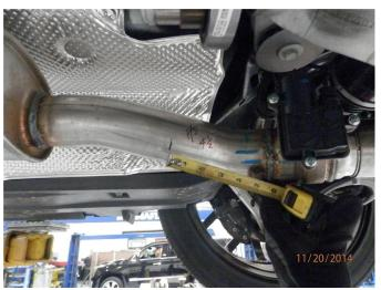
**Step 4.** For the passengers side cut 4.50" in front of the welded hanger forward of exhaust control valve as shown in the attached picture. With both valve assemblies cut from the OEM system, loosen the band clamps attaching the mufflers to the OEM tips. Both tail pipe sections may now be removed.
