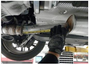
**Step 3.** For the drivers side cut 4.75" in front of the welded hanger forward of exhaust control valve as shown in the attached picture.
