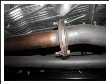
**Step 1.** To begin the removal of the OEM system you will need to remove the spare wheel. Next unbolt both inlet flanges at the OEM inlet ipie assembly. Working rearward (with the exhaust supported) extract the hangers from the rubber insulators and remove the OEM exhaust. Do not discard or damage the rubber insulators as they will be used to install the new exhaust system.
