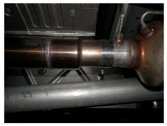
**Step 2.** There are two inlet pipe assemblies in the kit. 1. Wheelbase of 128.3" requires 6.5" Nipple. 2. Wheelbase of 140.5" requires 15.5" extension pipe and 6.5" Nipple. Begin installation of your new MAGNAFLOW system by loosely attaching the Inlet Pipe Assembly to the DPF outlet pipe you have just cut using the supplied 2.75" and 3.50" clamps. Engage the welded hangers to the rubber insulators.
