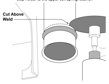
Cut away the bump stop holder immediately above the weld as illustrated. HINT: A die grinder with cut-off wheel or reciprocating saw is useful for cutting away the bump stop holder.
