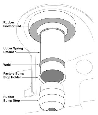
O Locate the factory weld that secures the bump stop holder to the upper coil spring retainer.
